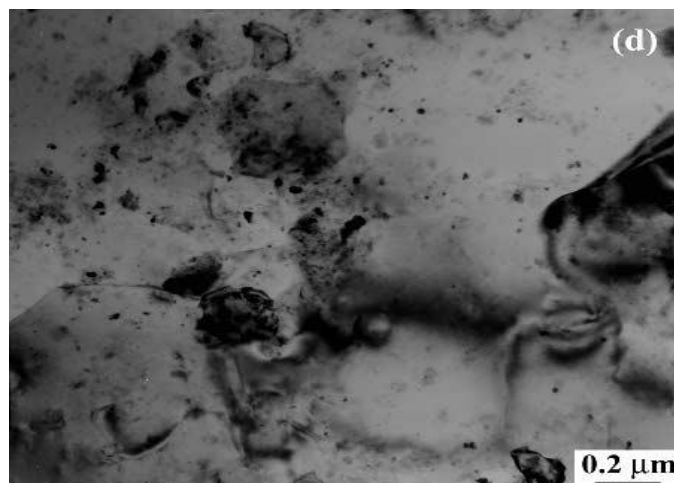
Figure 14: TEM micrographs showing (a) grains in as-extruded Al-4Mg-1Zr, and (b) Al 3 Zr particles in as-extruded Al-4Mg-1Zr, (c) grains in FSP Al-4Mg-1Zr and (d) Al 3 Zr particles in FSP Al-4Mg-1Zr
